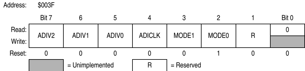
Figure 5-8. ADC Clock Register (ADCLK)
